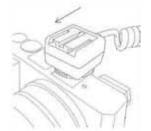
Reach M+ connects to the camera hot shoe port which is synced to the shutter.
