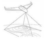
Sub-microsecond accurate photo time marks are stored in a raw data RINEX log during the flight.
