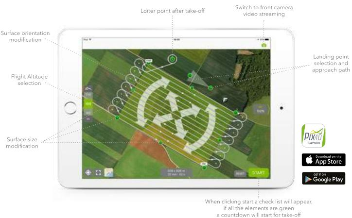
Pix4Dcapture is the easy-to-use flight planning mobile app that creates automatic and optimized flight plans to map a defined area from your mobile device.
